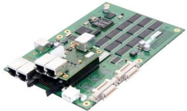
The power supply of the GLink-Splitter can be delivered in two different ways. One possibility is via a special power socket situated on the GLink-Splitter. The other is from the IE64\_HS board, in cases when the GLink-Splitter is plugged into the board.
